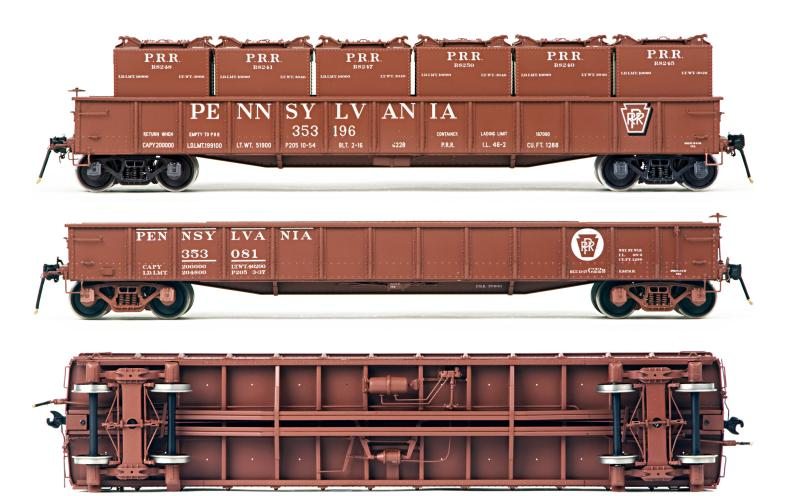
In the photos above you see elevation views of the car both with and without its container load. The containers that are shown in the photo are HB1a hopper-bottom versions. Also shown is the underside which lets you see the complete construction and running gear detail.
